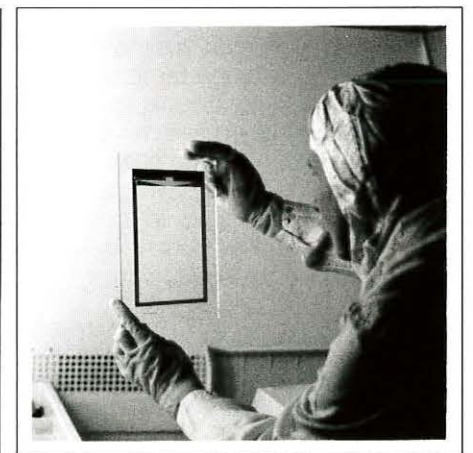
Fig. 2: Large high-precision masks for defining the electrode and active-element patterns in flat-panel displays can be made with a thin layer of chromium on a glass substrate. This technology, adapted from the integrated-circuit industry, is far more precise than the one based on a photographic emulsion and polymer film, which had been adapted earlier from the printed-circuit-board industry.
