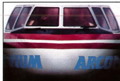
Indium Oxide Coatings help keep jet windows clear even under extreme temperature conditions.
